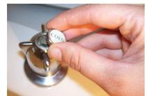
**Then pull off the handle** (the bit which turns). If there's a cover over the bottom of the tap, you'll need to take this off too. Wrap a cloth around it first so you don't scratch it, and undo it with a shifting spanner.
